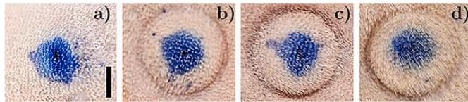
Fig. 5. Effect of applied load on GP skin (top view) supported by a layer of lean pork meat (*thickness* = 2 cm) after a jet injection of dyed water through a nozzle with an orifice diameter of  $155 \mu\text{m}$  for (a)  $L_n = 0 \text{ N}$ , (b)  $L_n = 4.9 \text{ N}$ , (c)  $L_n = 9.8 \text{ N}$  and (d)  $L_n = 19.6 \text{ N}$ . Scale bar represents 5 mm.
