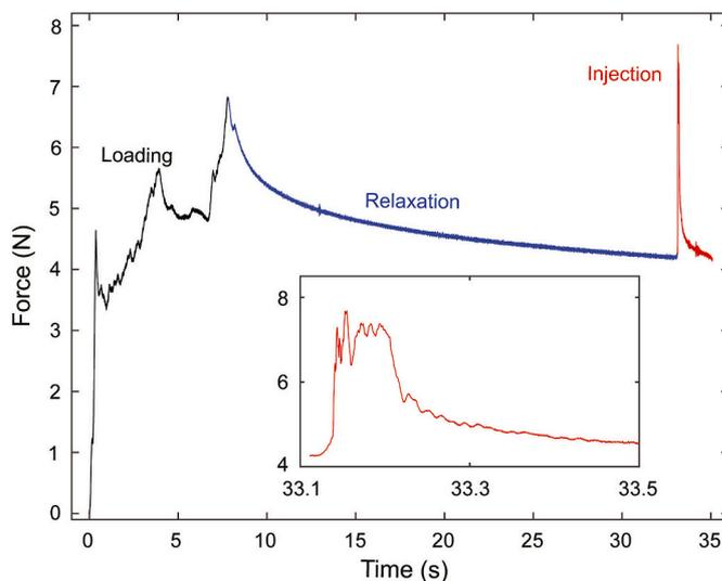
**Fig. 2.** Force measured by the load cell underneath the weighing balance plate for 80% glycerol solution injected through a nozzle with an orifice diameter of 155  $\mu\text{m}$  into the GP skin with  $S = 0$  mm and  $L_n = 4.9$  N. The different stages in the force profile include (i) the loading stage, (ii) the relaxation stage and (iii) the jet injection stage. Inset shows the force profile during jet injection.
