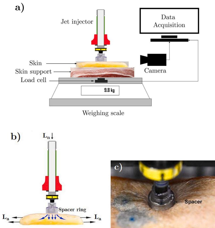
**Fig. 1.** Experimental. **a).** Schematic of the experimental setup, **b).** Schematics of applied normal load,  $L_n$  and axial load,  $L_a$ , both shown by black arrows, and hypothesized distribution of stress in the skin tissue shown by blue arrows and **c).** Human skin under tension by a spacer ring with an applied normal force load of 9.8 N by jet injector. (For interpretation of the references to colour in this figure legend, the reader is referred to the Web version of this article.)
