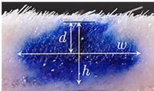
Fig. 3. The dimensions of the bleb formed inside the skin after jet injection.  $W$  is the maximum width of the bleb,  $h$  is the total depth of the bleb from the surface of the skin, and  $d$  is the distance between the depth at the maximum width of the bleb and the surface of skin.
