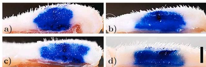
Fig. 6. Cross-sectional view of the blebs formed in the GP skin supported by a layer of lean pork meat (*thickness* = 2 cm) injected with dyed water ( $V = 100 \mu\text{L}$ ) through a nozzle with orifice diameter of  $155 \mu\text{m}$  for (a)  $L_n = 0 \text{ N}$ , (b)  $L_n = 4.9 \text{ N}$ , (c)  $L_n = 9.8 \text{ N}$  and (d)  $L_n = 19.6 \text{ N}$ . Scale bar represents 5 mm.
